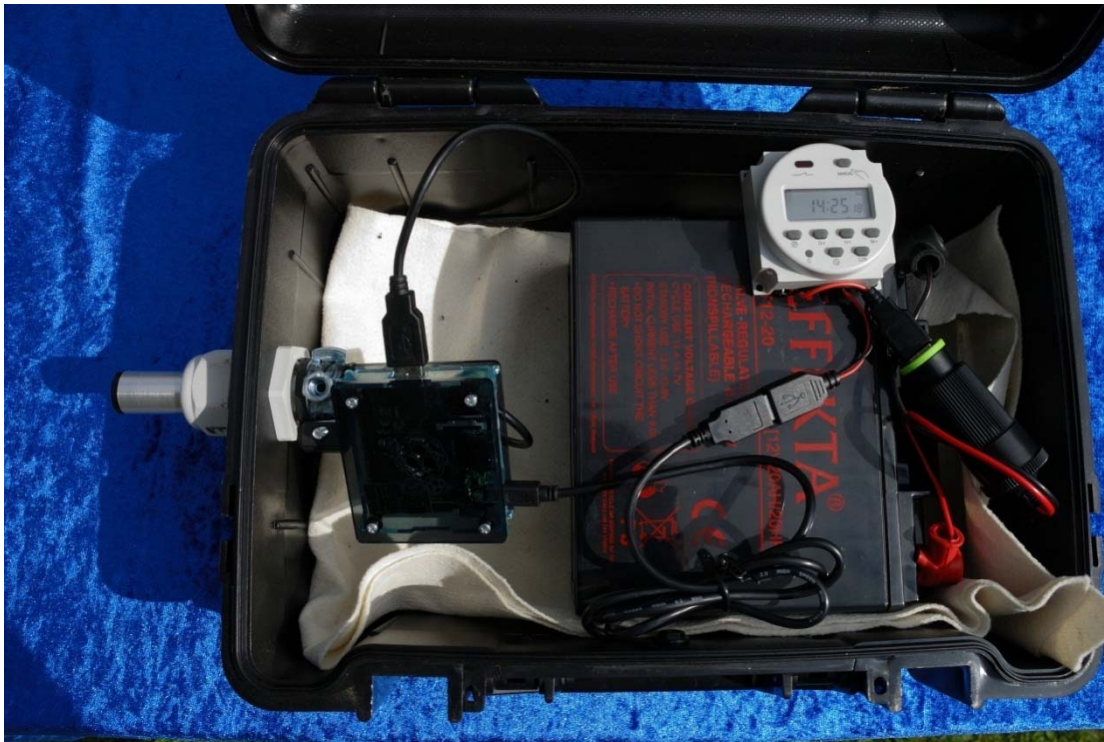
Model A+ with 20 Ah lead-acid battery, cottenpickers clock timer, Belkin voltage converter 12/5 Volt and Dodotronic Ultramic250K in a water-resistant XCASE
