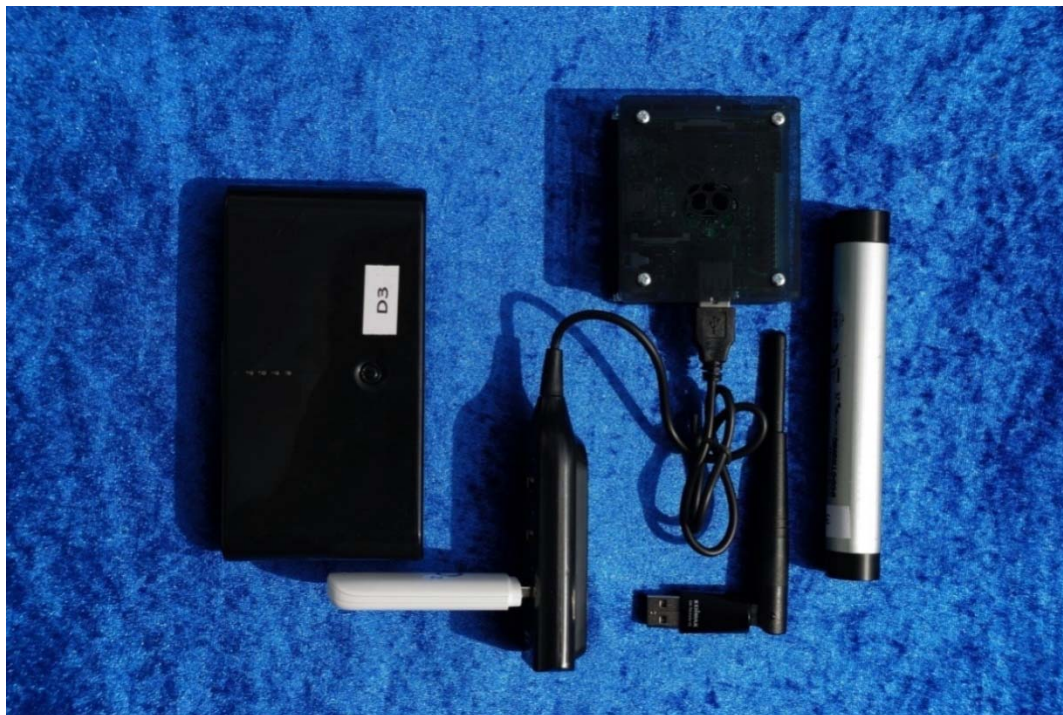
Model B+ with accumulator (Dadidong), WLAN antenna (Edimax),UMTS stick (white, Huawei Model E173u-1) and Dodotronic Ultramic250K
