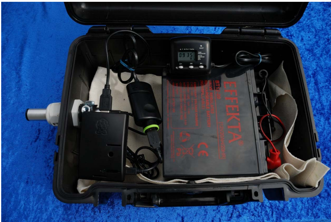
Model B+ with 20 Ah lead-acid battery, 12 Volt weekly timer, Belkin voltage converter 12/5 Volt and Dodotronic Ultramic250K in water-resistant XCASE
