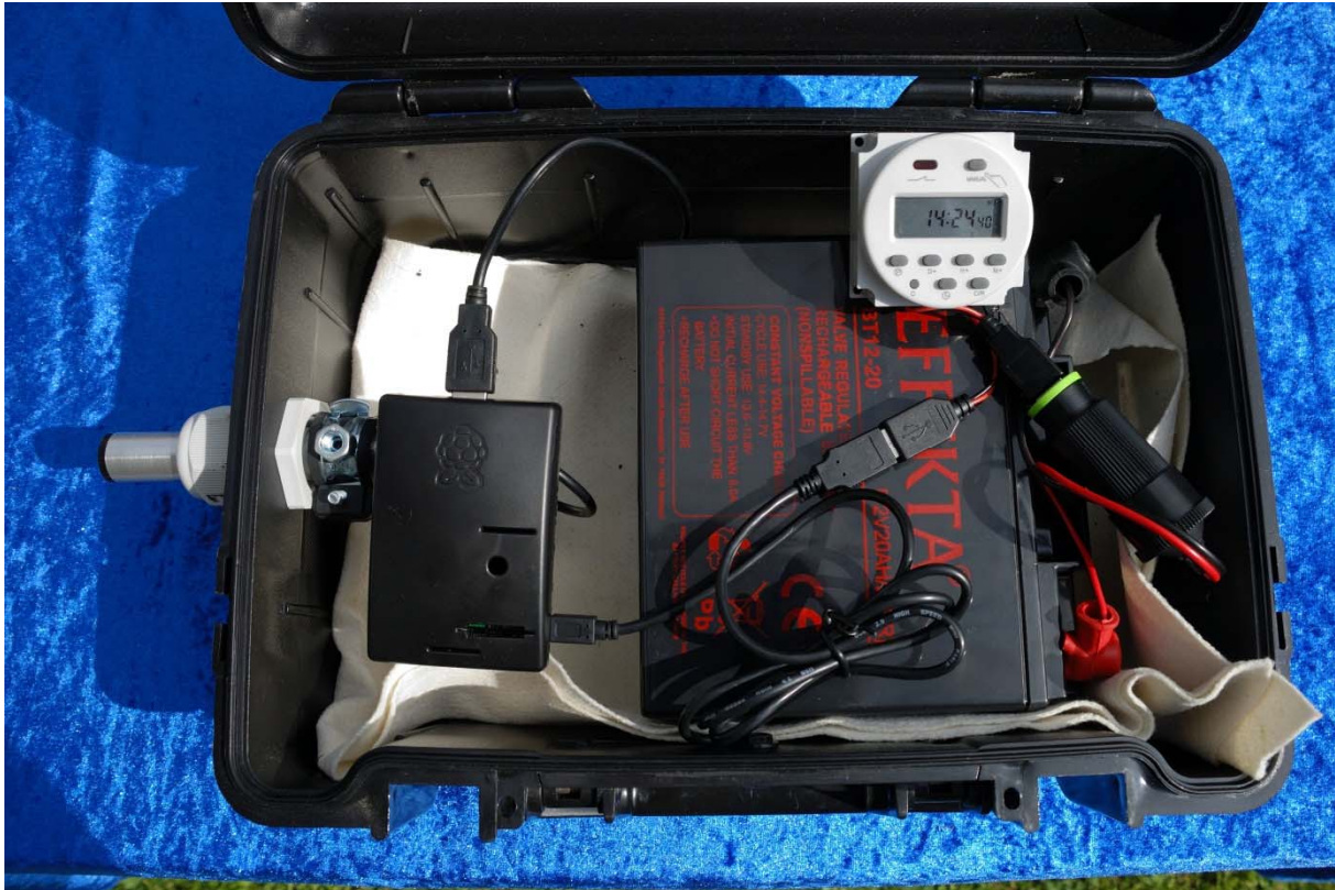
Model B+ with 20 Ah lead-acid battery, cottonpickers clock timer, Belkin voltage converter 12/5 Volt and Dodotronic Ultramic250Kin water-resistant XCASE
