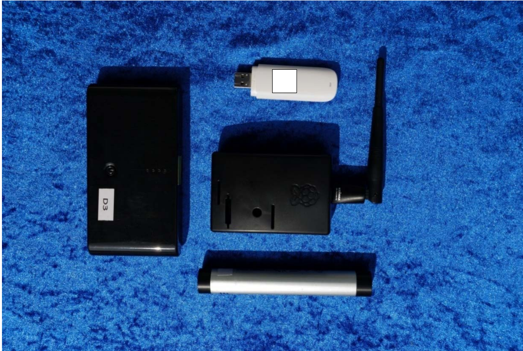
Model B+ with accumulator (Dadidong), WLAN antenna (Edimax),UMTS stick (white, Huawei Model E173u-1) and Dodotronic Ultramic250K
